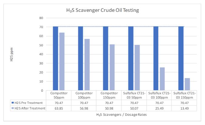
The acceptable efficiency rate for H2S scavengers is **4-5** ppmv Scavenger / ppmw H2S at maximum value. The results show that the **Competitor** Product, while somewhat effective, is above this value (**7,55**). On the other hand, the product **Sulfaflux CT21-03** has an average efficiency value of **2,30**, which is well below the acceptable threshold.
