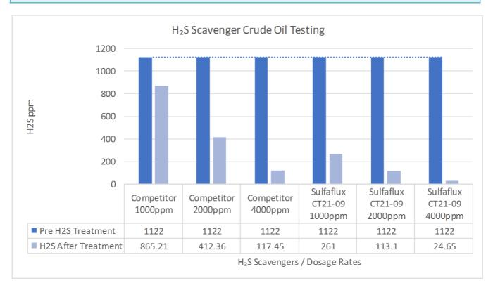
The acceptable efficiency rate for H2S scavengers is **4-5** ppmv Scavenger / ppmw H2S at maximum value. The results show that the **Competitor** Product, while somewhat effective, averages **3.57**. On the other hand, the product **Sulfaflux CT21-09** has an average efficiency value of **2,26**, which is well below the acceptable threshold.
